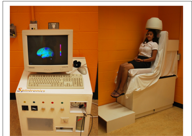
FIGURE 1 | The mock neuroimaging device assembled from discarded odds and ends including a scrap salon hair dryer. Throughout the mock scan, a pre-recorded video displayed rotating three-dimensional brain slices with accompanying scanner-like audio, lending the appearance of collecting and analyzing patterns of brain activity.
